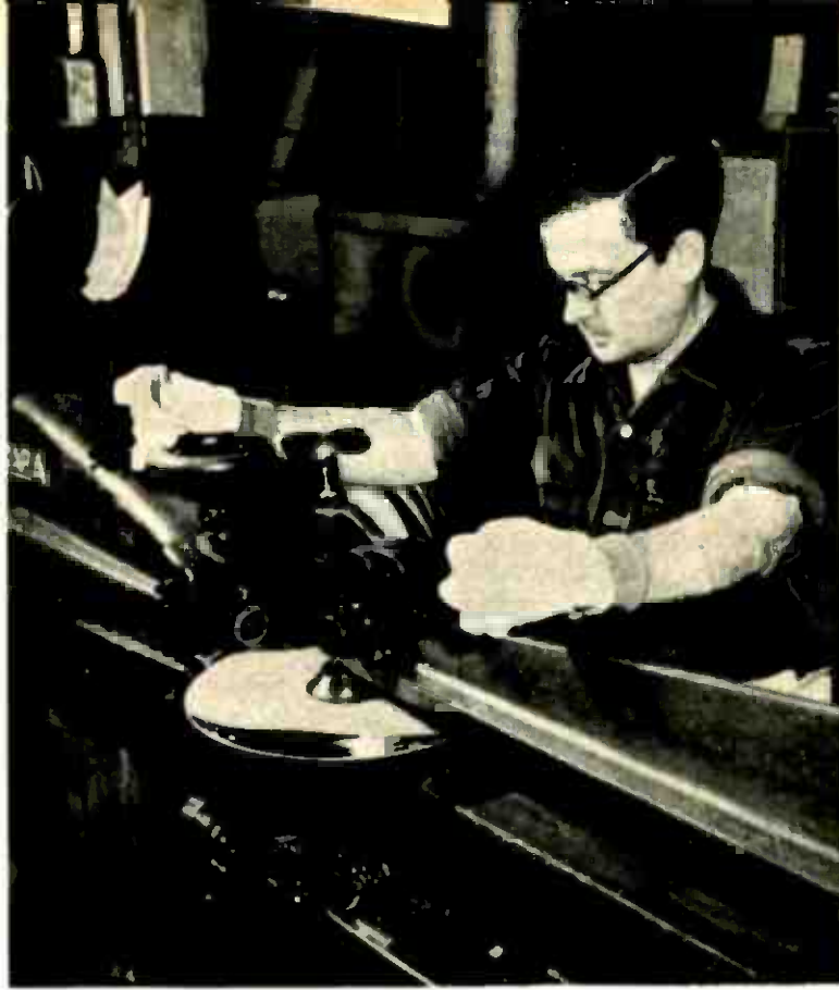
2. A mold is then made from the master disc. Here the mold is being carefully separated from the master. Each step in record-making calls for utmost precision
