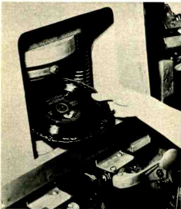
5. The pressed disk is inserted in dinking dies for trimming, as shown in the picture above, after which it is inspected for imperfections
