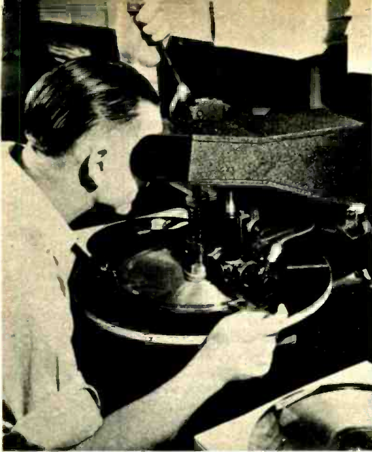
3. From the mold, a nickel stamper is made for pressing records. In order to center the stamp accurately, the operator shown above is using a microscope
