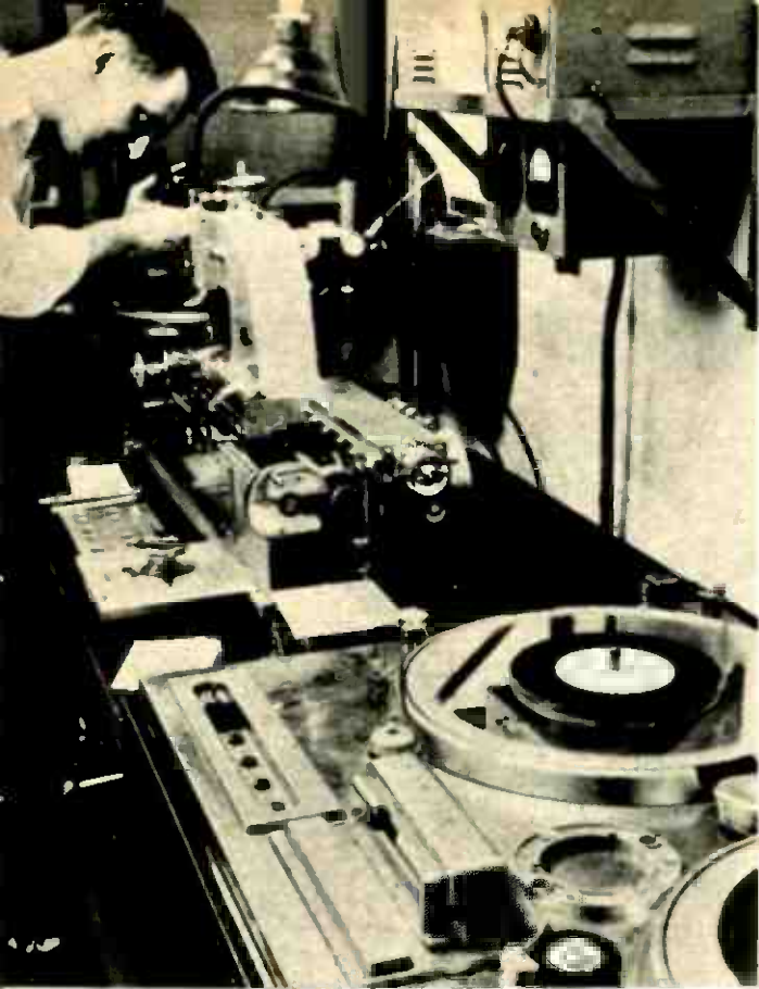
1. Steps in making a record: A recorded tape is being re-recorded on a master disc. Electric impulses cut grooves in the plaster surface of the record
