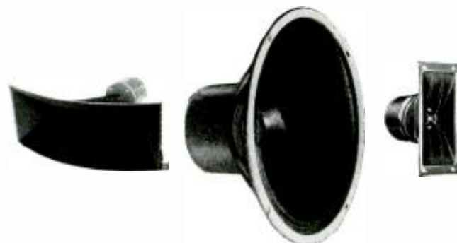
Fig. 6. Tweeter horns capable of reproducing down to 600 or 800 cycles are too large for use in coaxial units. Therefore, crossover in coaxials is often above cone-breakup frequency.
