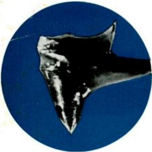
Above: Enlargement of so-called "bargain" stylus. (Unretouched photo)
