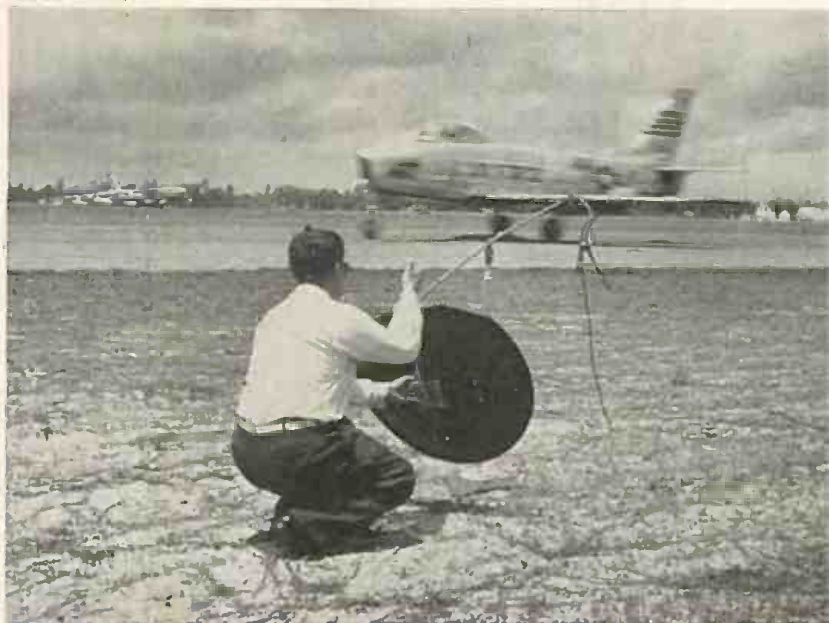
Lt. Col. Hugh Day tracks an F-86 with parabolic microphone.
