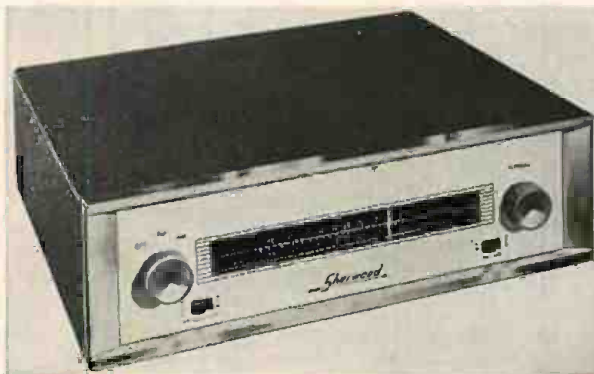
The S-2000 has AFC, flywheel tuning.
