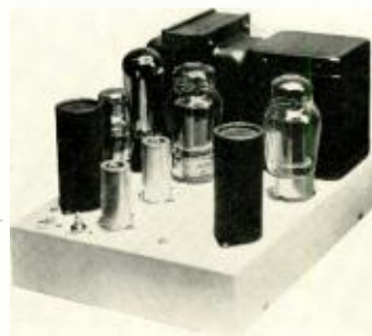
A-340A amplifier uses 100-watt 6550's.
