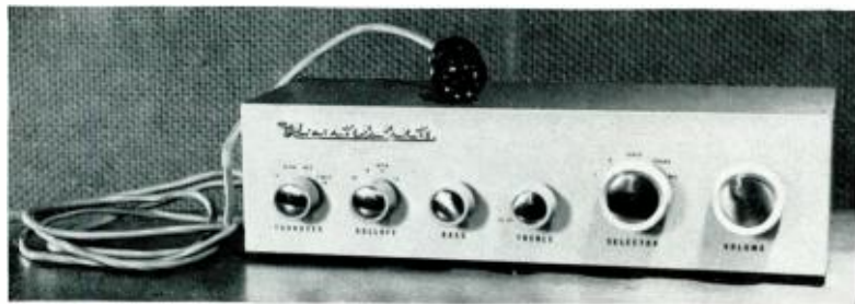
Heathkit WA-P2 preamplifier-equalizer-control unit obtains power from amplifier.
