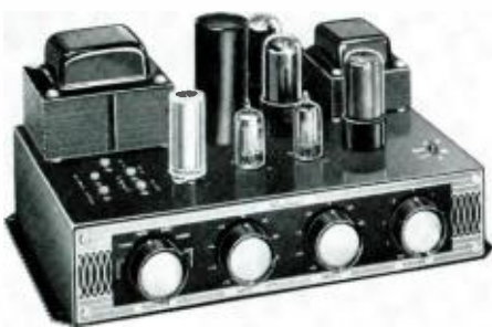
Low-cost Rauland amplifier includes preamp and control sections.
