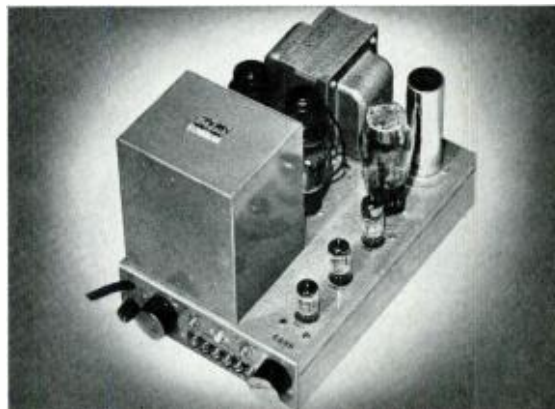
Amplifier can put out full 30 watts at any audible frequency.
