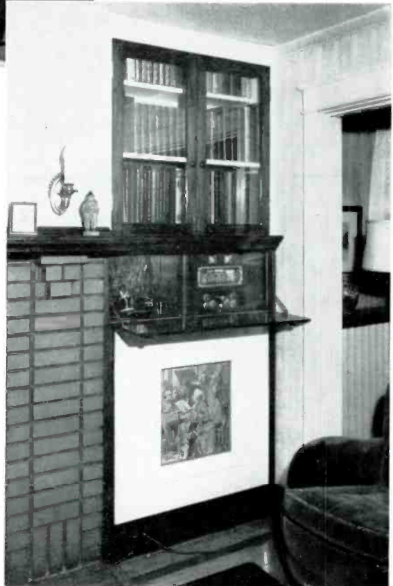
The Prades, a fine modern piece by Balladier. A combination FM-AM tuner, control unit and 12-watt amplifier is used, and a Webster player with a GE cartridge. Speaker is a separate unit.
