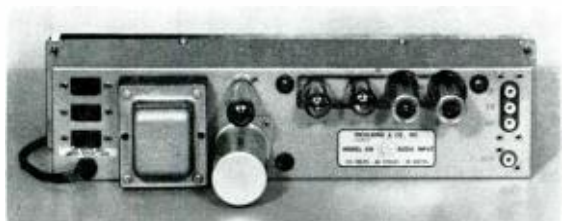
Five tubes are used in this preamplifier. Four are shock-mounted.
