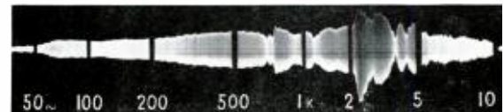
Fig. 19. Axis response of 8-in. unit mounted in wall of test room forming true infinite baffle.
