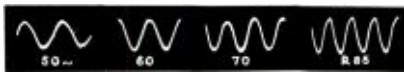
Fig. 13. Tapered pipe. Microphone 12-in. from open end. As with reflex loading, the low frequency wave shape is better at the open end of the air chamber than it is at the cone, a phenomenon which helps to improve general quality.
