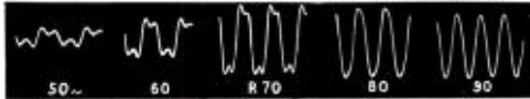
Fig. 11. True infinite baffle. It is very interesting to note the distortion at the cone resonance (70 cycles). As the frequency is lowered, the amount of distortion remains the same, but the intensity of the fundamental frequency goes down until a point is reached where the harmonic content is as great as the fundamental, and the output contains 50% of frequency doubling. If the frequency is taken still lower, a point can be reached where the fundamental disappears and only harmonics are heard, producing a "knock" instead of a note. It is quite obvious that a speaker with a low cone resonance is required for good results here.
