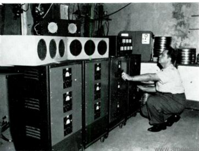
Checking volume levels on recording-and-mixing amplifiers at sound laboratory maintained by Cinerama at Oyster Bay, N. Y.
