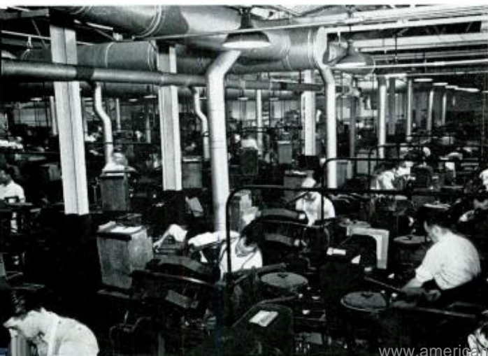
Record-press room at EMI's Hayes plant. More shellac than vinyl is processed, owing to big export business to "backward" areas.
