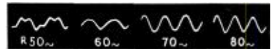
Fig. 7. The output level from the small H-R cabinet is rather low, but the waveform is quite sinusoidal at 70 cycles. There is of course distortion at the lower cone resonance at 50 cycles. The upper resonance occurred at 100 cycles but was free from distortion. Corner position as in previous tests. See Fig. 16 for effect of increasing the input to 2 watts. The performance is far superior to the reflex cabinet A, which is 40% larger.
