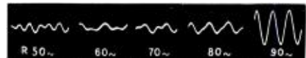
Fig. 4. Poor results from 8 in. unit in small reflex cabinet A. Note low level of output and poor waveform below 90 cycles. Upper cone resonance occurred at 110 cycles. Corner position as Fig. 3.
