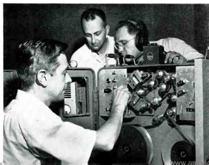
Film follows devious track in playback machine. Technician at right is hearing seven mixed channels via binaural earphones.
