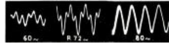
Fig. 3. 8 in. unit on 3 x 2 ft. 6 in. baffle placed in a corner of test room. Note severe distortion at 72-cycle resonance and enormous drop in output level at 60 cycles compared with Fig. 11.
