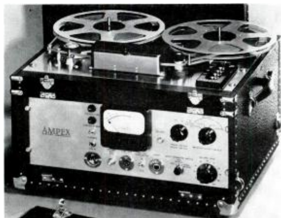
Professional tape recorder and playback unit operates at 7\frac{1}{2} or 15 inches per second, has three heads, pushbutton control, and accommodates 2500 feet of tape on standard 10-inch reels.
