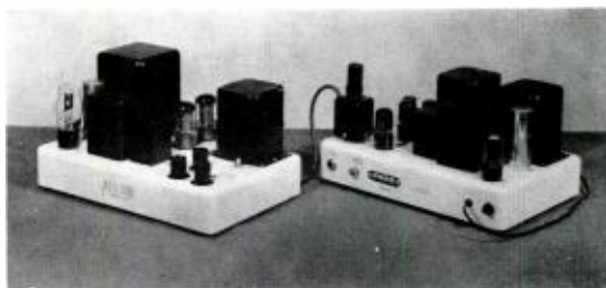
Dual system employs two amplifiers: a 25-watt for amplification of low frequencies (left) and a 10-watt unit of similar design (right) to carry the high frequencies. Note crossover network, plugged into left-hand corner of high frequency chassis.
