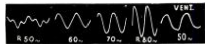
Fig. 5. Greatly improved results from larger reflex B with much louder output. Upper resonance now occurs at 80 cycles. Note the very good waveform at 50 cycles from the vent. Corner position as Figs. 3 and 4.
