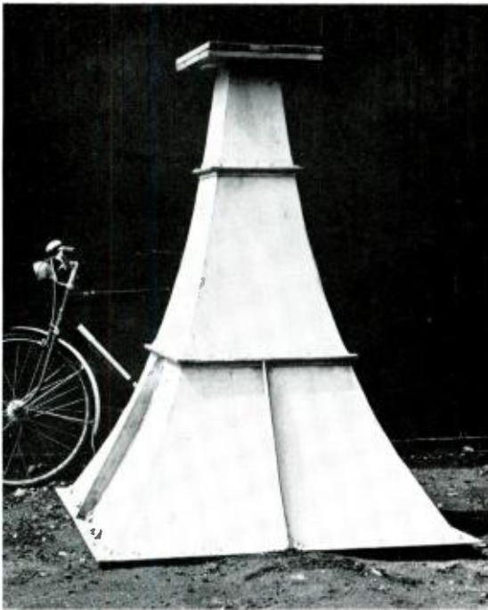
Fig. 2. Exponential horn used, with bicycle to indicate size.
