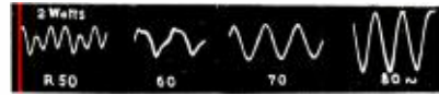
Fig. 16. Small H-R. The effect of increasing the acoustic output by using 2 watts is shown here, and should be compared with Fig. 7. The distortion at 50 and 60 cycles is of course increased, but the quality is still very good at 70 cycles; it is in fact superior to the small reflex A at half the acoustic output.
