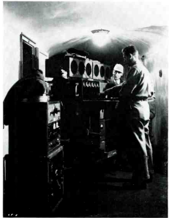
Mobile recording unit, by Reeves for Cinerama. Only real multiple recording, so far, has yielded convincing stereophonic results.
