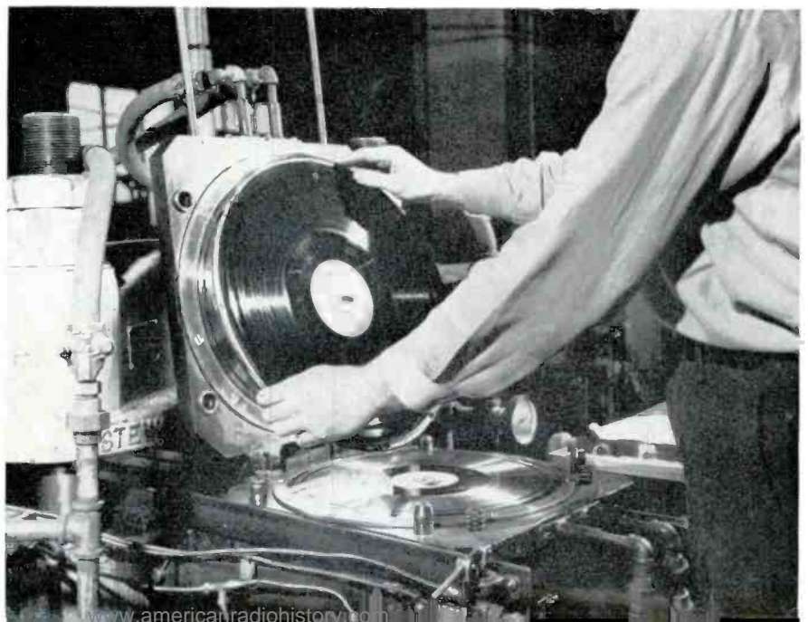
MOLDED TRANSCRIPTION: When the press is closed, the Vinylite material is heated and subjected to 1,800 to 2,000 lbs. pressure. A cycling control releases the press after 25 to 75 seconds, depending upon the size of the disc and the kind of material being molded. Excess material is squeezed out around the edges. Therefore, the final operation is to trim and polish the circumference of the disc. Since the labels are molded onto the disc during the pressing operation, the disc is ready, after it is trimmed, to be packed and shipped.
