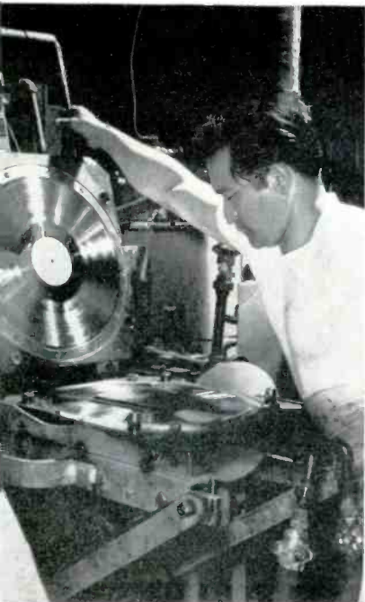
PRESSING: Two matrices are mounted in the press. Then a preform of Vinylite is put between the stampers, and the press is closed.
