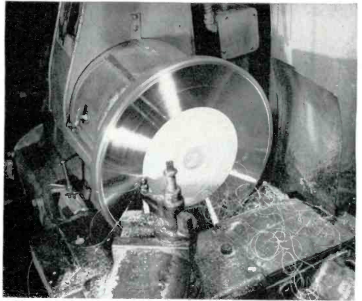
BACK TURNING: The back of the matrix must be ground or turned perfectly smooth, since any high spots in the plating would deform the matrix during the pressing operation.
