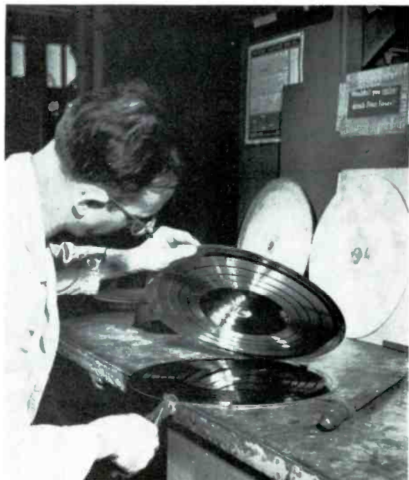
STRIPPING: The matrix is finally stripped off the master record, disclosing a bright gold or silver surface that is an exact negative copy of the record grooves. Great skill is required in this operation.
