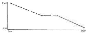
7. This is the frequency response curve of a record compensator. It is the exact opposite of that shown in sketch 5.
