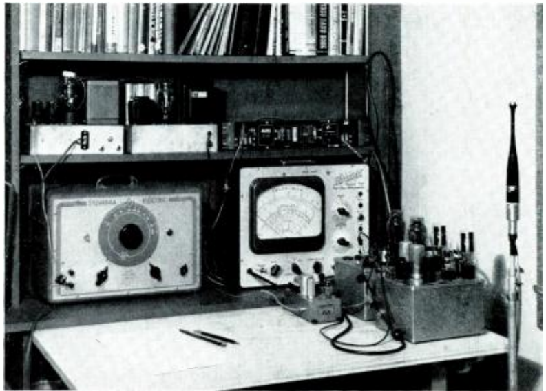
Fig. 4. Equipment used to test frequency response of experimental Air-Couplers included a Sylvania audio oscillator which was fed into the Williamson-type amplifier, directly above it in the illustration. Power supply for the Altec 21-B microphone is shown to the right of the Williamson. The microphone (moved near the equipment for photographic reasons) was connected to a Pickering preamplifier, which was modified to remove bass compensation circuits. This, in turn, was fed into the McIntosh 50-W-2, at right on desk. Output of the 50-W-2 was measured on the Hickok V'TV'M.
