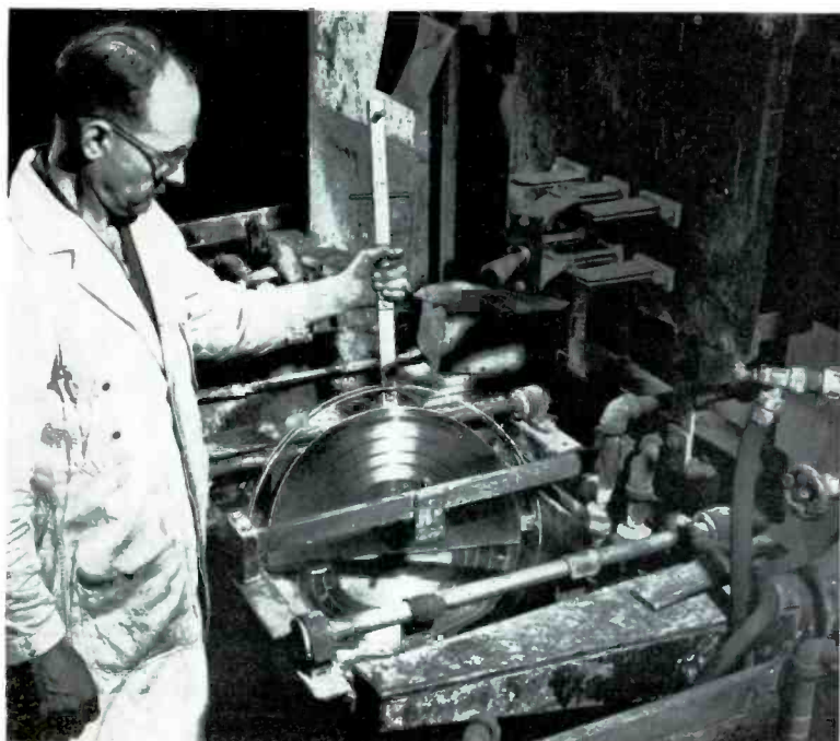
ELECTRO-CLEANING: After stripping, the matrix is cleaned thoroughly by immersion in a strong alkaline solution, agitated by an electric current. In this way, impurities can be removed without damaging the delicate negative copy. One particle might cause a click when the record is played.
