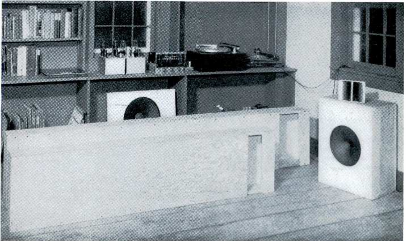
Fig. 12. Temporary arrangement used during experiments with 15-in. speakers shows both 6-ft. and 8-ft. Air-couplers.
