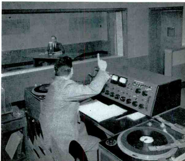
Dual transcription turntables and control equipment at WQXR
