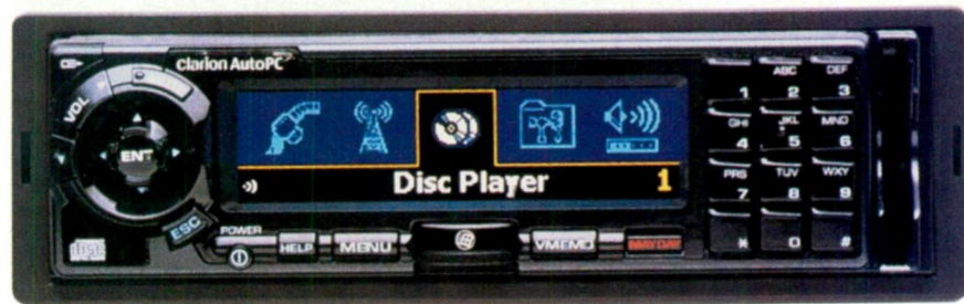
Clarion's AutoPC ($1,299) was designed in partnership with Microsoft. The single-DIN-size head unit is not just a CD receiver but a multifunction in-car computer.
