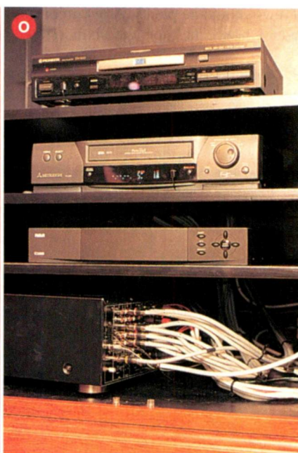
N. Cook makes the final connections to the Yamaha A/V receiver. O. With all of the audio and video cables in place, the receiver is ready to be positioned on its shelf inside the cherry wall unit that was custom-built for the new system.
