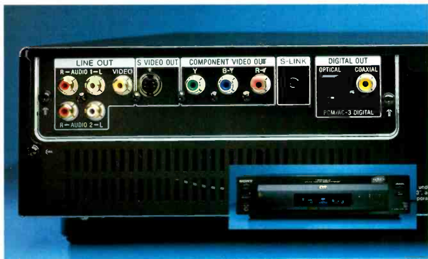
The rear panel of Sony's DVP-57000 DVD player shows the wide variety of audio and video outputs that may be provided on a company's flagship model.
