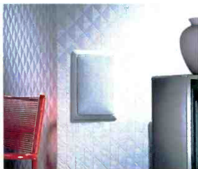
Boston Acoustics' Model 350 ($300 a pair) has a 5¼-inch woofer and is rated down to 68 Hz. Installation requires a 9 x 6-inch cutout and 2½ inches of rear clearance.
