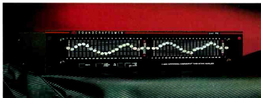
MTX Soundcraftsmen's E440PRO twenty-one-band graphic equalizer ($549) has one-third-octave spacing from 40 Hz to 1 kHz and variable spacing from 1 kHz to 16 kHz; the boost/cut range is 15 dB per band. Its C-MOS switches are said to reduce noise and distortion.
