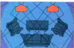
Bose Direct/Reflecting® speakers accurately reproduce live music's natural balance of direct and reflected sound energy, in full stereo (blue area) throughout the room.
