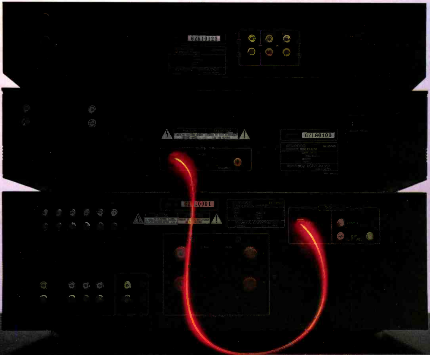
We removed the protective coating from the cable shown to clearly illustrate a fiber optic transmission.
