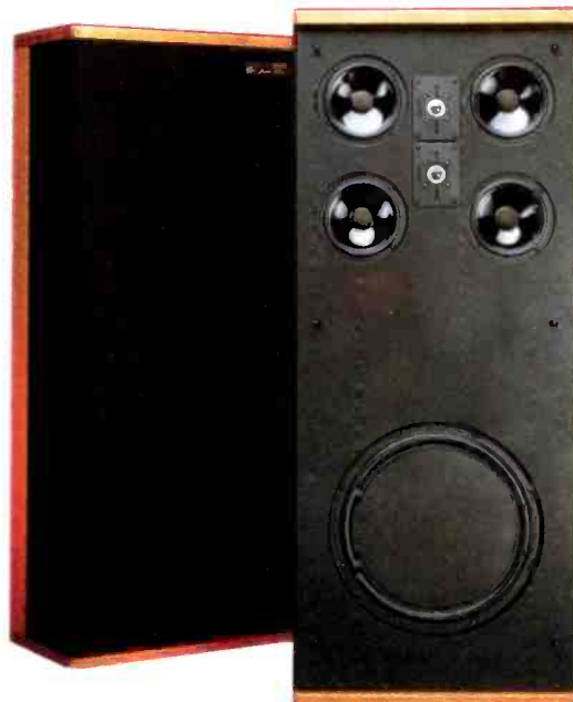
Each SDA-SRS-2 speaker (below) from Polk Audio in Baltimore reproduces part of the other channel's signal, but out of phase, in order to cancel interaural crosstalk and improve imaging.
