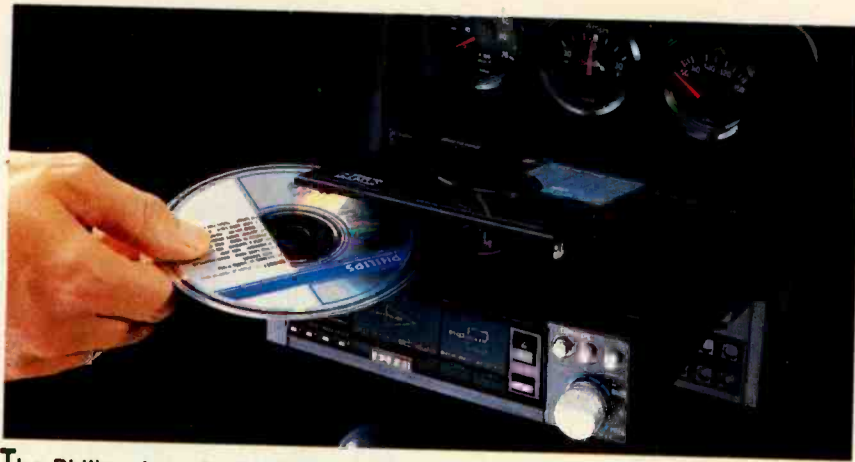
The Philips Auto Audio CD10 ($550) pops out of the dash for use as a home or portable CD player, or just to protect it from theft.
