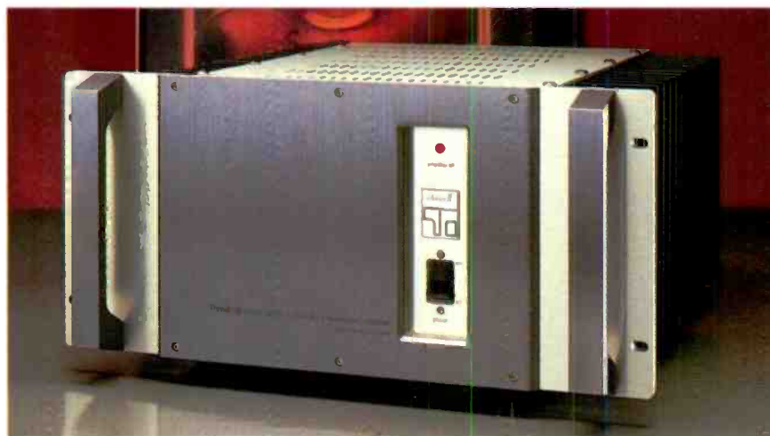
The pure Class A power amplifiers from Threshold, in Sacramento, California, utilize Nelson Pass's Stasis technology—which is also licensed to Nakamichi in Japan. Stasis amplifiers, like the Threshold Model S/500 shown below, use no negative feedback, and their performance is virtually independent of load characteristics, signal dynamics, and spectral content.
