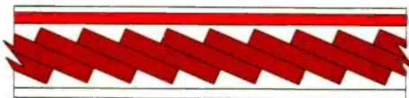
On new hi-fi stereo videocassettes, sound is recorded across nearly the entire width of the tape, using methods which allow simultaneous recording of video within the same area.
