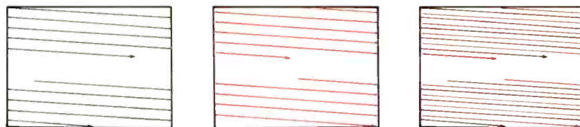
Figures 1a (left) and 1b (center) show how a video frame is scanned in two separate fields. Figure 2 (right) shows the scan lines interlaced to form a complete image.
