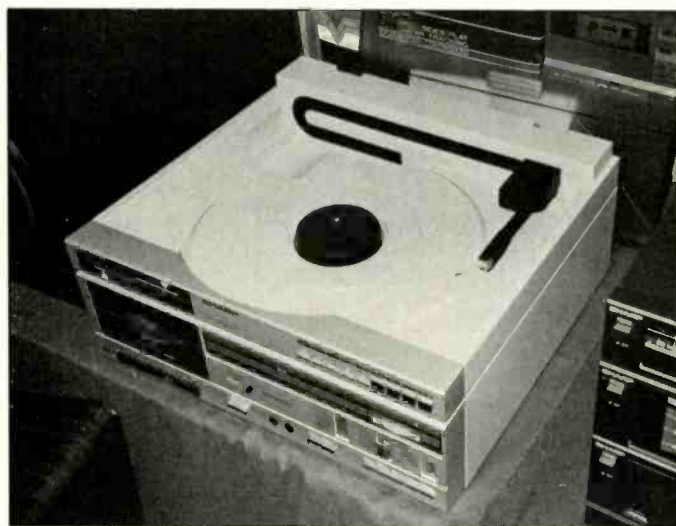
Above, the tone arm in Sharp's RP-117 turntable makes a hairpin turn in order to play both sides of an LP without flipping the record over. Price: $249.95. Right, Custom Woodwork & Design has a drawer for storing Compact Discs. The drawers will fit all CW&D audio cabinets; each stores seventy-five CD's and costs $70.
