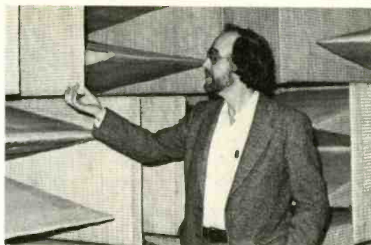
Checking out fiberglass wedges in an anechoic test chamber
