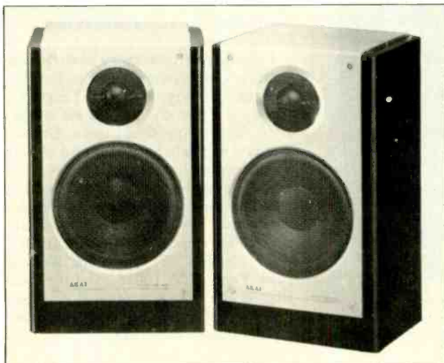
Both the Akai AE-63 (left) and Bose 301 Series II (above) are designed to take advantage of reflected sound. The AE-63 has a tweeter and woofer up front and a tweeter and passive radiator in back. The Bose unit has a second tweeter directed to the back.
