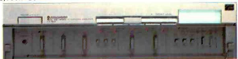
With the glass door closed, your preset controls are protected while you select your program source and volume.
