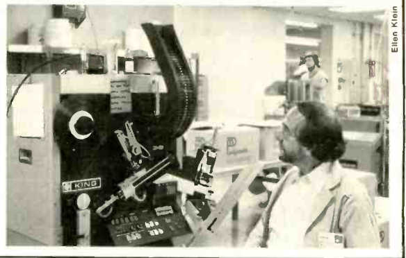
Technical Director Klein watches as cassette tape ("pancake" at left) is loaded into empty shells.
