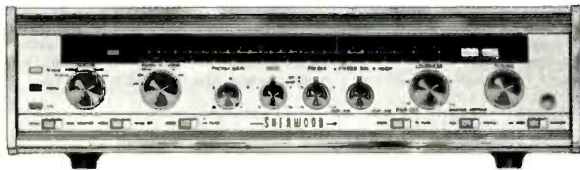
Suggested retail price (1963) $374.50. S-7700 II AM/FM Receiver. 36 watts RMS per channel. Analog flywheel tuning. 21 tubes, 16 diodes.
