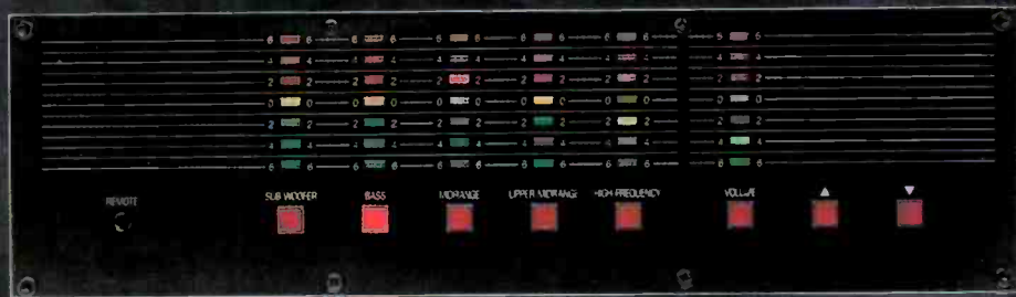
An LED control panel adjusts the levels of 5 separate amplifiers in each speaker cabinet.
