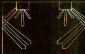
The drivers in a 301 speaker pair are positioned asymmetrically for a more natural balance of reflected and direct sound energy.
