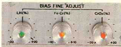
Bias Fine Adjustment allows precise fine tuning for optimum response.
