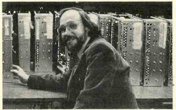
Technical Director Klein fingers some naked chassis stacked for inspection on Sherwood's assembly line.
