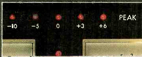
5 LED peak level indicators help eliminate distortion.
