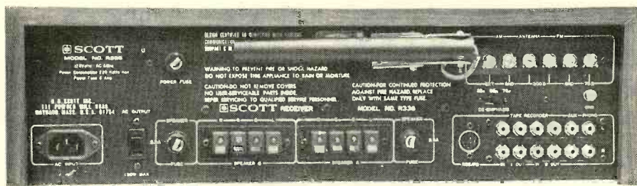
The R336's rear panel has spring-loaded connectors for speakers, screw terminals for external AM and FM (300 or 75 ohms) antennas, and a detachable power cord (socket at lower left).
