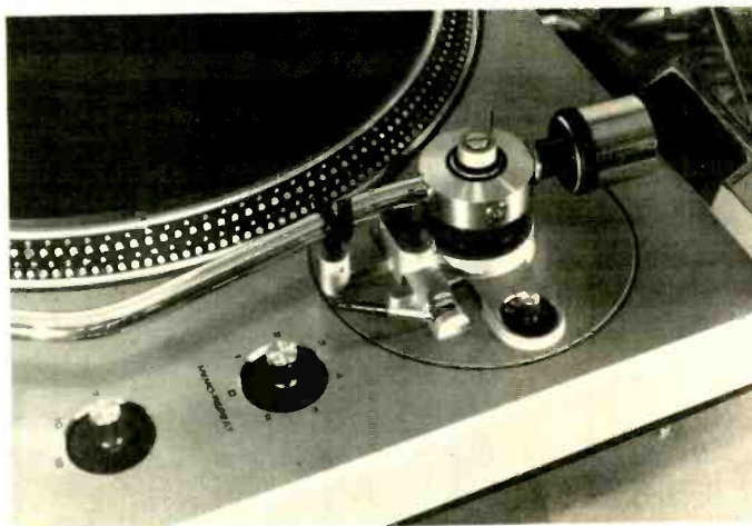
The tone-arm pivot assembly of the SL-1300, with anti-skating adjustment to the side and the MEMO-REPEAT selector further to the left.
