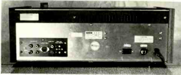
The Teac 450's jack panel is quite simple, consisting of inputs and outputs (via phono jacks or DIN socket) and Dolby calibration controls. Switched a.c.-accessory outlet is at right.
