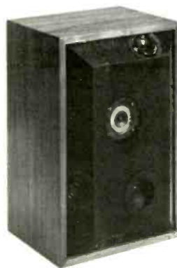
The D-6 with grille removed, showing the five tweeters (four on the sloping edges, one facing forward) and the mid-range with dispersion-enhancing radiation aperture. The rear-mounted woofer is protected by a sturdy perforated screen.
