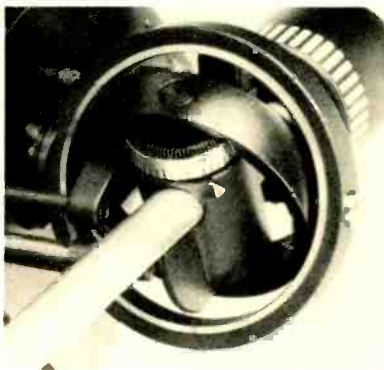
Gyroscope twin-ring gimbal of Dual 1229 and 1218 tonearms. Tonearm pivots vertically along axis of inner ring; horizontally along axis of outer ring. All four suspension points have identical low-friction needle-point bearings.
