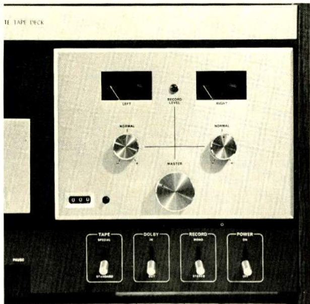
The SCT-6's two smaller knob controls are used for initial balance of the two recording channels; the large master knob then serves to adjust levels of both channels simultaneously.
