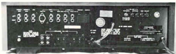
The SX-727's three pairs of speaker outputs accept the special plug-in connectors supplied with the receiver. One of these is shown in place, without the speaker leads attached.
