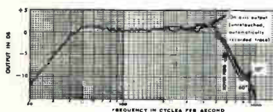
Frequency response of the AR-3a 12-inch woofer, radiating into a 360° solid angle (hemisphere).
