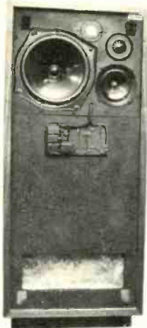
The four drivers in the IMF Studio speaker are closely grouped at the top of the enclosure. Elements of the crossover network are visible just below them, with the port at the bottom. In the more recent version tested, the crossover is internally mounted.
