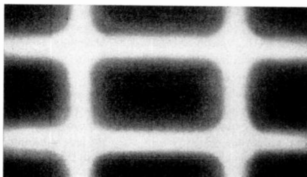
Fig. 3. Overhead view of sound-pressure distribution when the combined second-order resonance of a room's length and width is stimulated. Nine columns of maximum sound pressure result.
