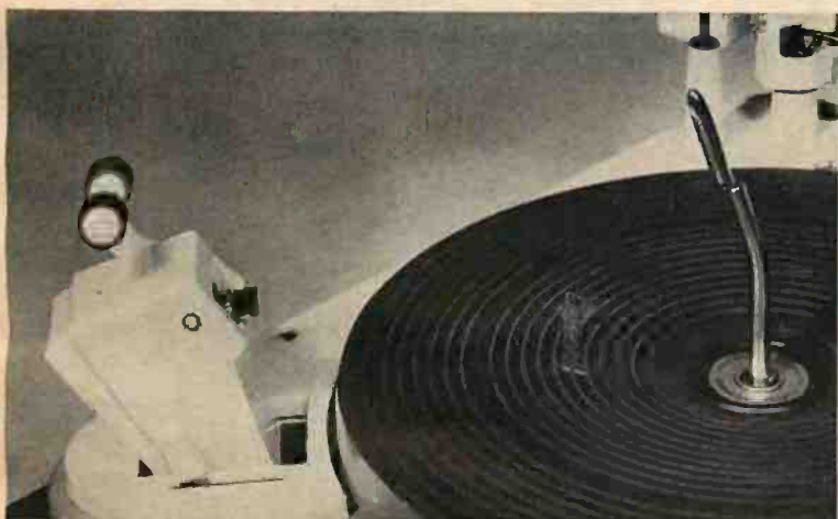
Pusher-platform type of changer mechanism allows records to drop of their own weight, and it has no moving parts in spindle.
