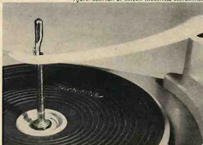
Straight center-spindle mechanism with overhead guide arm permits user to intermix records of different sizes.
