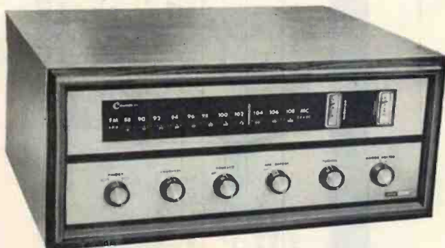
Harman-Kardon's Citation III employs two separate meters: one to indicate the signal strength, the other for center-channel tuning.
