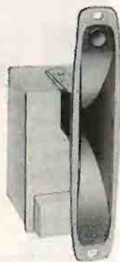
DuKane's Ionovac tweeter utilizes ionized air to create sound. ($79.00 with cabinet)
