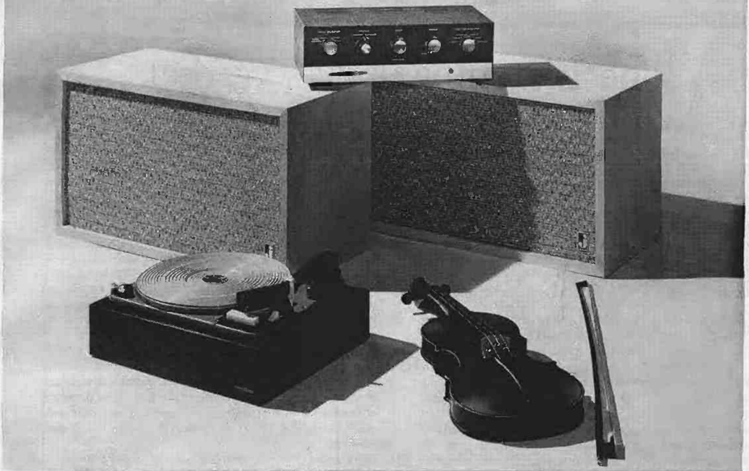
System No. 2. Components: Jensen TF-3 speakers, Heath WSA-2 stereo amplifier, Dual-1006 record changer with Pickering Stereo 90 cartridge. Total system price: $355.40.
