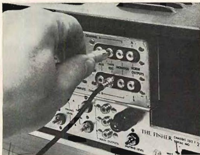
Connecting cables from the preamp to the recorder. To the right of these connections are those for monitoring, and the outputs feeding from the recorder to the hi-fi system preamp.
