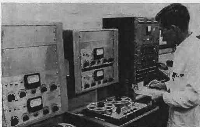
An engineer monitors the re-recording of a master tape to a ½-inch master duplicator. The wider tape insures highest fidelity, plus more strength and longer life.
