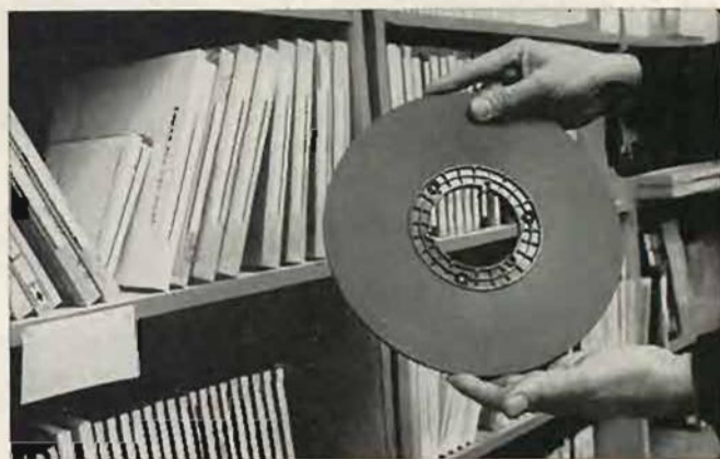
A pancake of \frac{1}{4} -inch 1-mil raw tape on a hub ready to be placed on a slave. Its 3,750 feet can provide more than 3 hours of recorded 4-track hi-fi stereo music.
