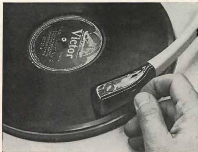
A convenient-to-operate record player is a must in dubbing old records. Choose one that comes up to speed readily, has a stop switch, and has a finger grip on the cartridge shell.
