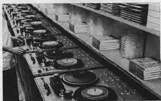
A master duplicator whirling at 120 ips feeds this bank of slave units operating at 60 ips. All four tracks (forward and reverse) are recorded simultaneously.
