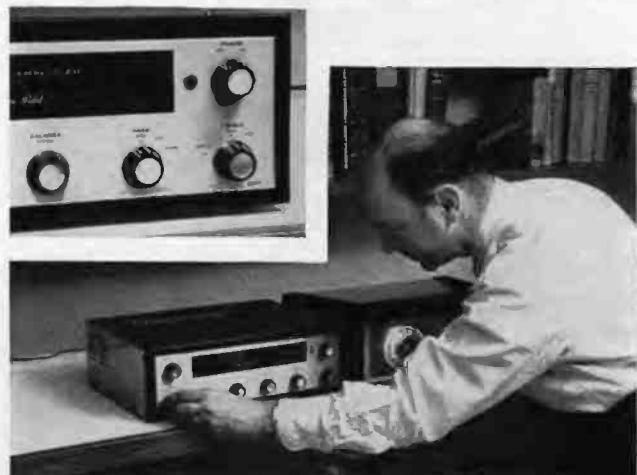
Pilot SM-244 features continuously variable record compensation through adjustment of the tone controls. Off and on rotary switch and jewel lamp are situated in the upper right hand corner of the attractively finished cabinet.
