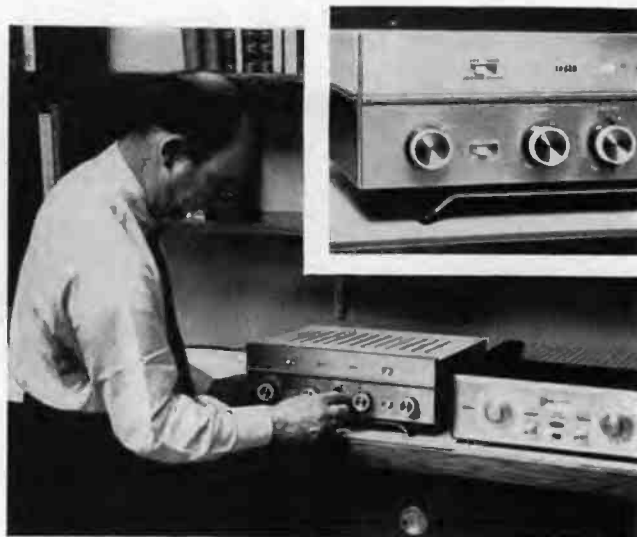
Bogen DB-212 has provisions to reverse speaker phasing of the second channel. Not all tapes and records are stereophonically recorded in the same phase. Bogen is the only manufacturer featuring this important item.
