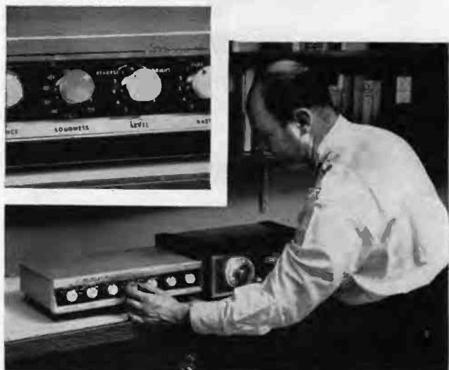
Four functions are combined in the Bell 3030 Loudness and Level controls. The former pulls out to turn set on and off and rotates to compensate loudness. The latter reverses channels and simultaneously adjusts level.
