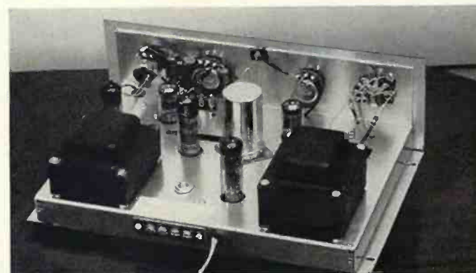
After going all out on high wattage amplifiers, Heath has released its 12-watt bookshelf amplifier Model EA-2, which uses five miniature tubes. The whole amplifier kit was wired in just under five hours. See review on page 60.
