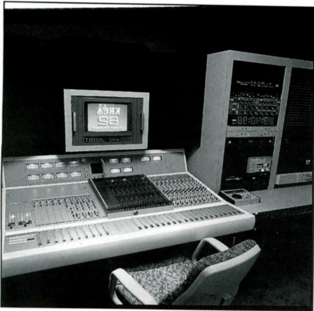
Figure 1. The Audio control room #2 at KRCA-TV, Burbank, located back-to-back of its companion Video Control room, is equipped with a 24-input Neve Series 55 mixing console.
