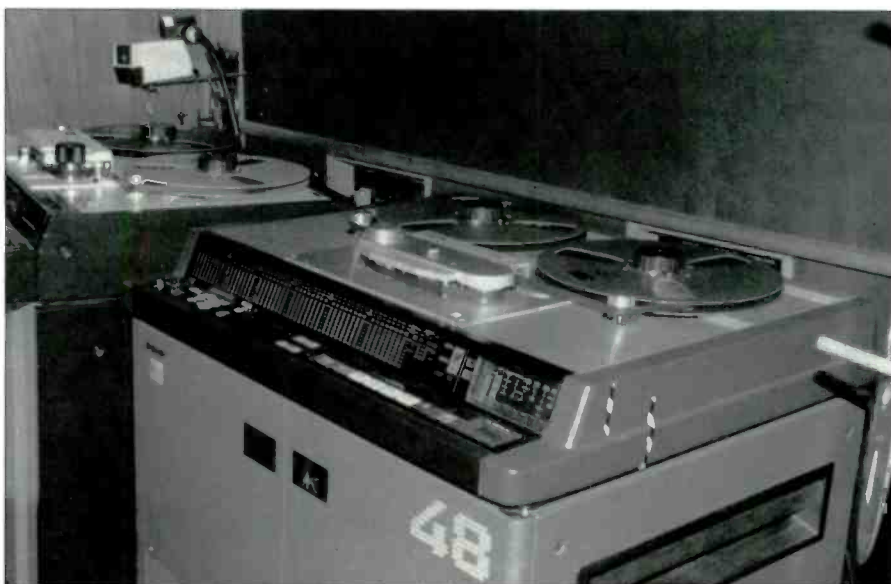
Figure 5. One of the Studio's Sony 3348s alongside a 3324 permit an entire production to be built up in the digital domain.
