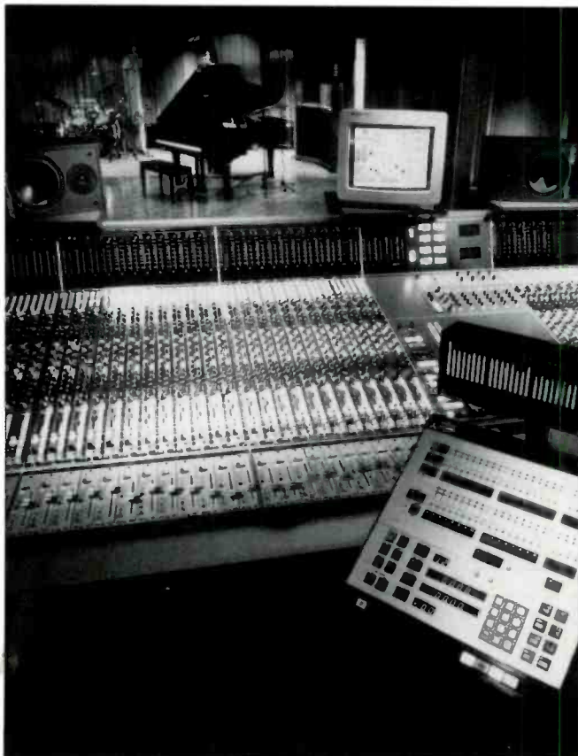
Figure 4. Studio B control. The Neve VR60 with Flying Faders are seen with a Mitsubishi 32-track digital recorder.
