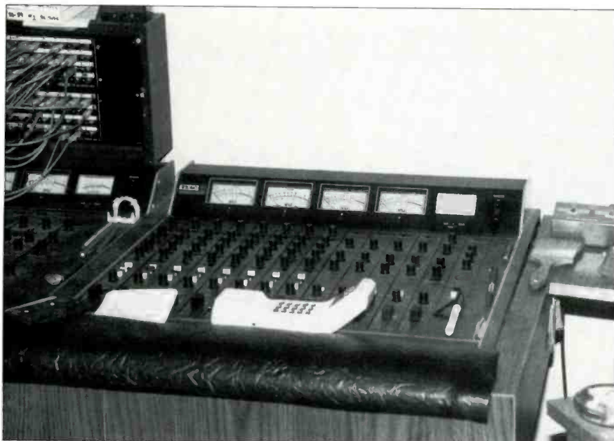
Figure 2. Two Tascam Model 5A consoles are bridged together to form a 16 x 8.
