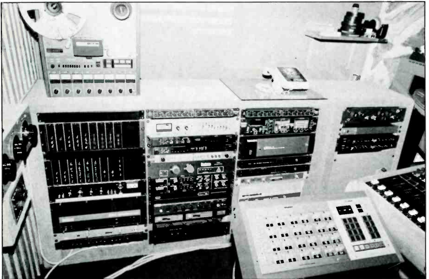
The equipment rack are in reach just to the right of the console. Note the Studer 24-track remote box in the foreground.
