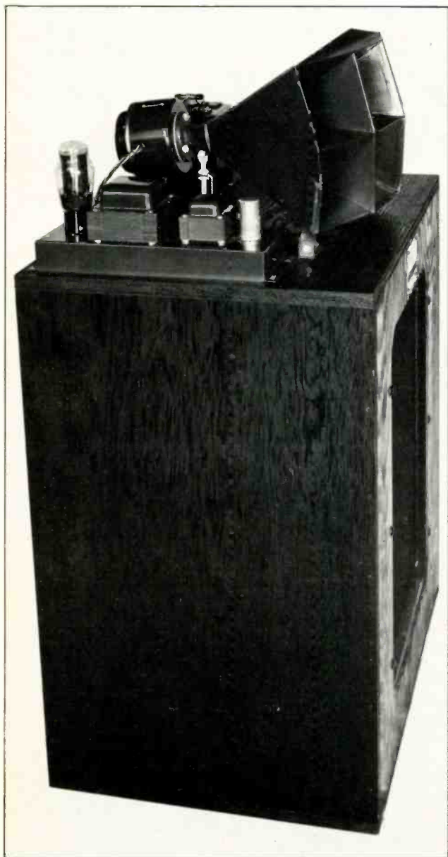
Figure 1. The Iconic monitor system. Built by Lansing Mfg. Co. during the '30s. Note power supply on top for powering magnetic field coils.
