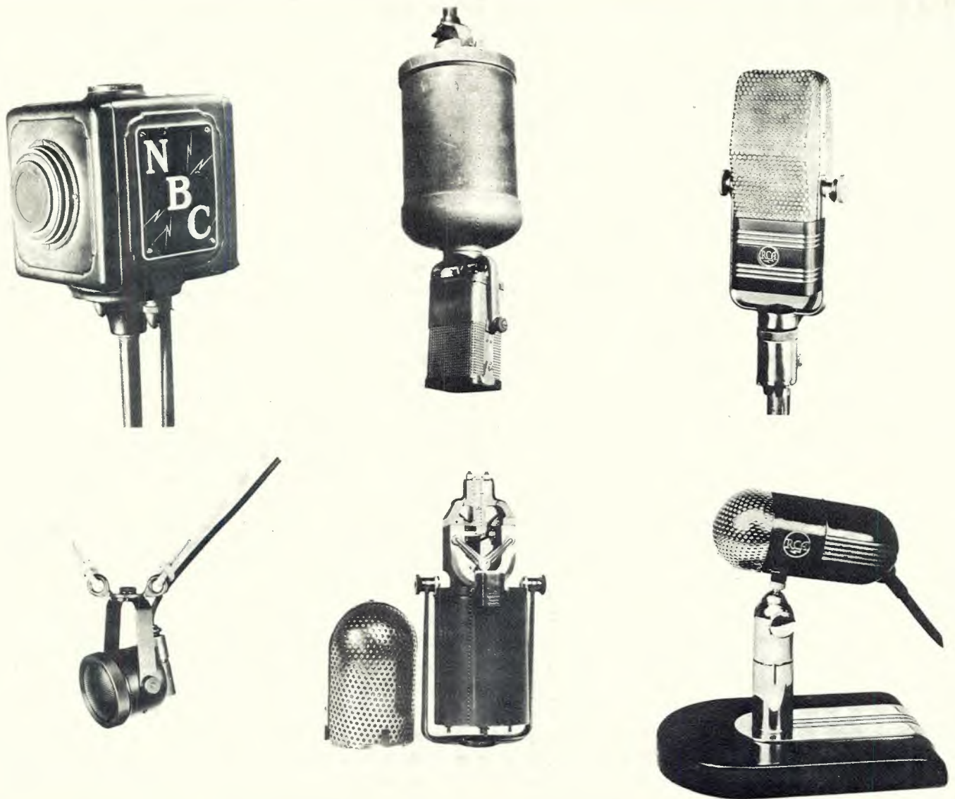
The ribbon mic has played a prominent role in the history of microphone design. Note the four ribbon microphones among these six early RCA mics. Top row, left: an early condenser type—1928; Center: an early modern ribbon microphone (velocity type)—1930; Right: The 44-BX velocity mic—1932. Bottom row, left: the model 50-A pressure type mic, first in the line of induction mics—1933; Center: the type 77-A universal (ribbon) microphone, forerunner of the present day 77-D—1936; Right: the 88-A pressure type mic.
