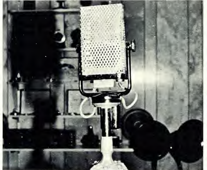
Figure 7. An RCA prototype ribbon microphone, circa 1931.
