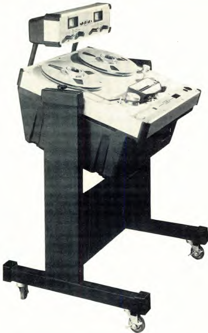
The Enertec Schlumberger F462 Super Stereo analog recorder.
