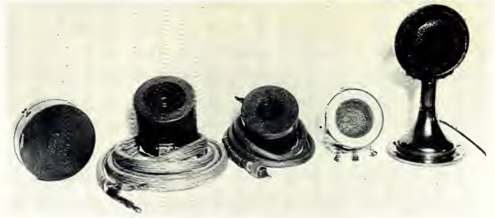
Figure 5. A collection of early Westinghouse microphones. From left to right: glow discharge, push-pull condenser, standard condenser, double-button "tomato can," and a double-button carbon mic in a special desk stand.
