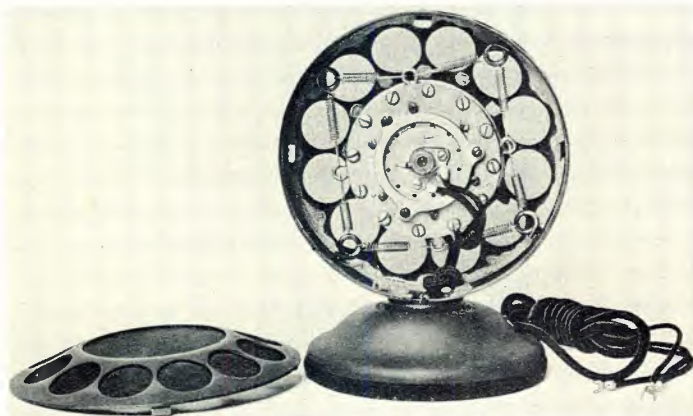
Figure 3. An improved "Acoustic Aparatus"; the Western Electric double-button carbon transmitter.
