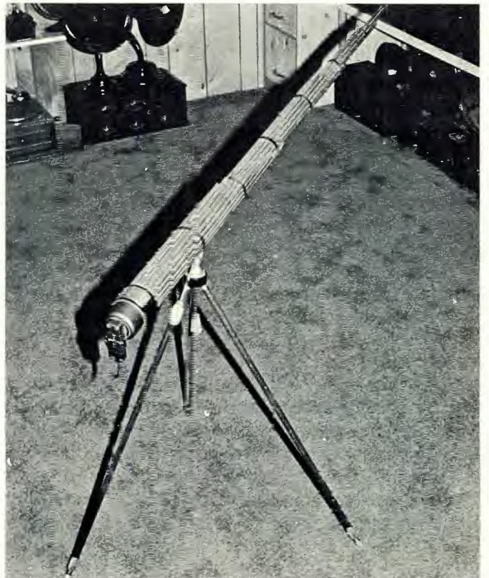
Figure 8. A Western Electric Shotgun microphone, circa 1937.
