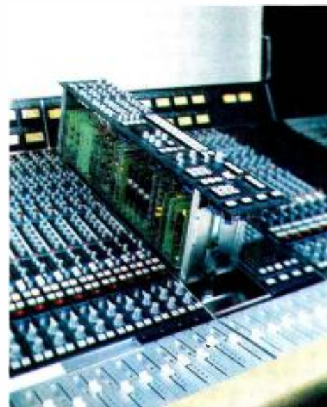
The SSL master panel, shown here in its raised position, contains echo return controls, quad output compressor, plus monitoring and cue controls.
