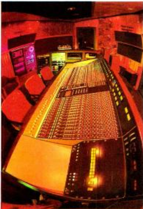
Solid State Logic's "super console"—recently installed in Kendun's new Studio D. This is the first SSL board to be placed in an American Studio.
