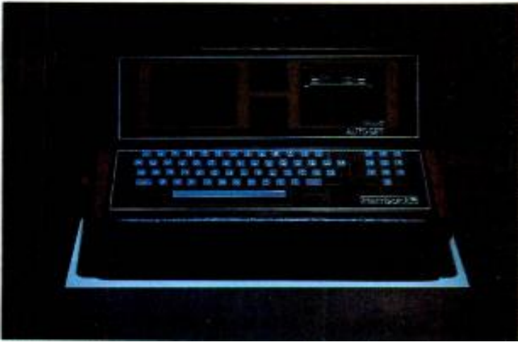
Figure 1. The main systems housing of Harrison Systems' Auto-Set. Above the keyboard are a five-inch CRT monitor and the data cartridge drive system.
