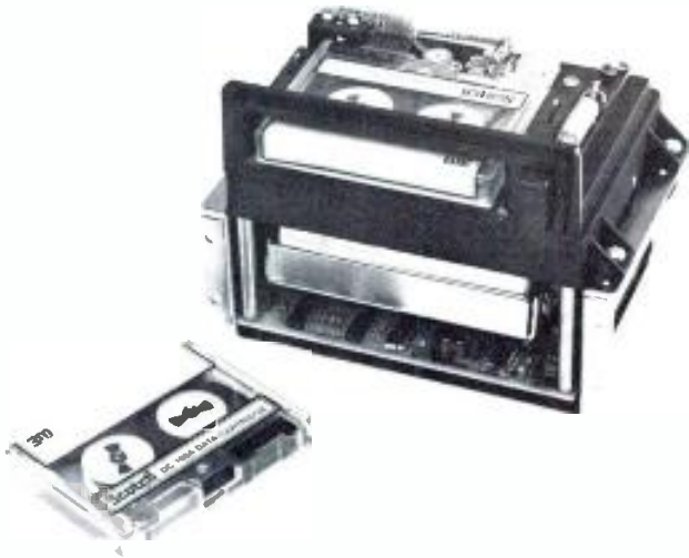
Figure 1A. The 3M DC-100 data cartridge and its drive system.
