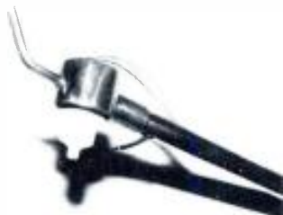
The vacuum head. A nylon thread acts as a buffer between the disc and the head. It is slowly sucked off a below-deck reel into the bottle with the dirty fluid.
